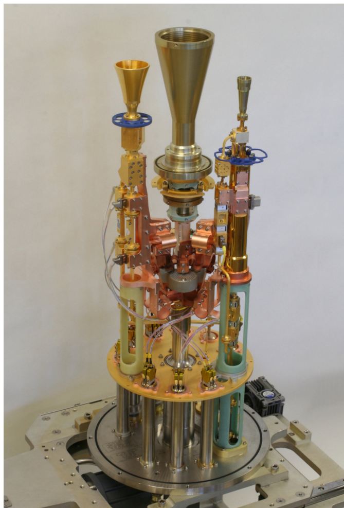
Fig. 2 The cryogenic LNA assembly with the vacuum dewar removed. The 7 mm band horn and low noise amplifiers are on the left, the 12 mm band horn and low noise amplifiers in the centre and the 3 mm band horn and low noise amplifiers on the right
