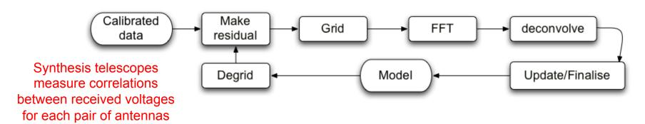
To the first order (narrow FOV), the measurement equation is a 2D Fourier Transform
