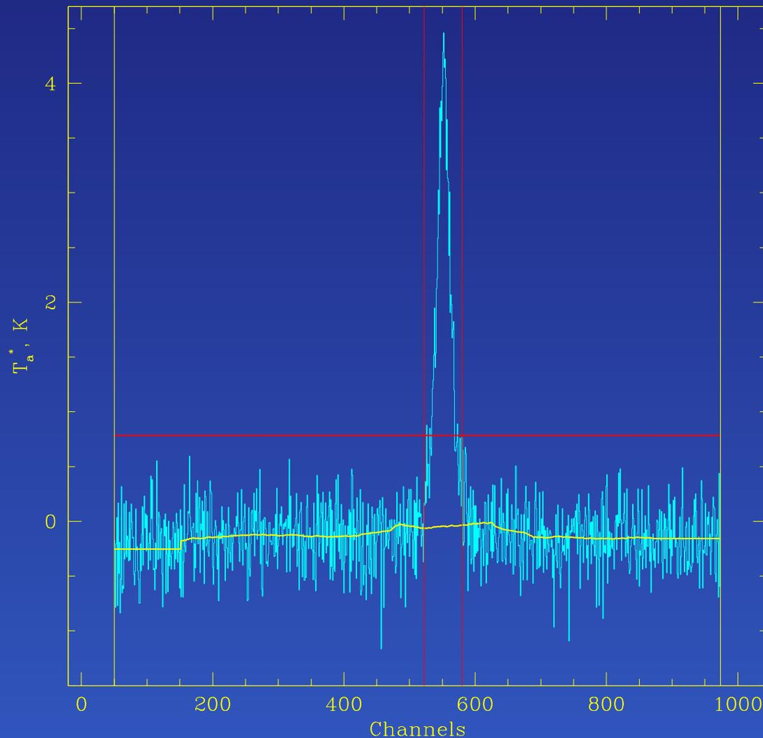
For this Mopra spectrum, the algorithm with the rejection of 50 channels from each side and  $3\sigma$  detection limit finds the line at **522–580** channels
