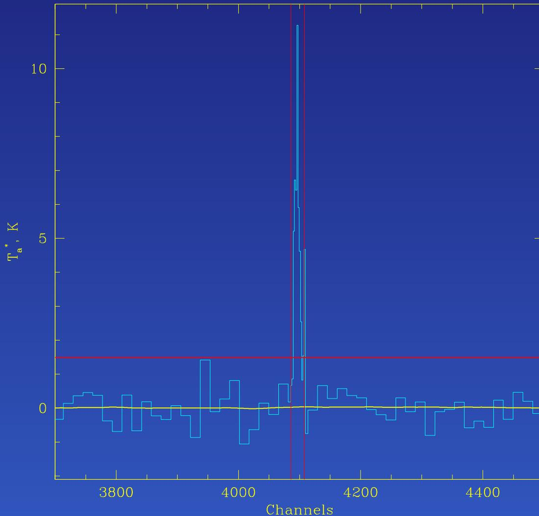
For this spectrum, the algorithm detects a line above the  $3\sigma$  detection limit at **4086–4108** channels. Averaging of adjacent channels is necessary here to reveal the line.
