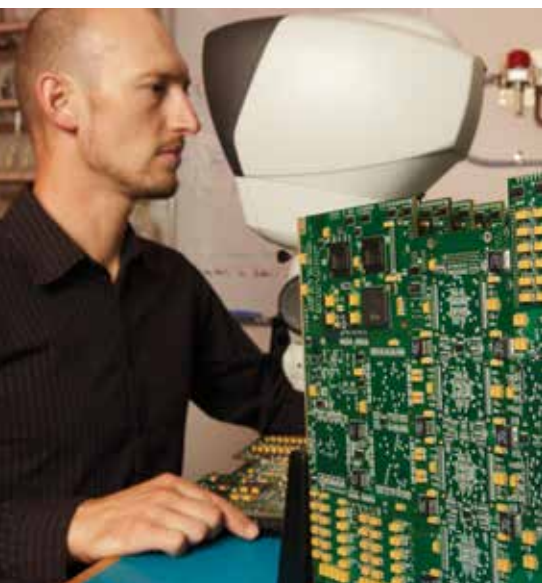
Signal processing boards built by CSIRO for a recent upgrade of the Compact Array. Photo: Tim Morison.
